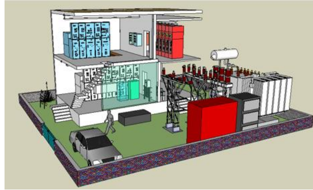
Compact 33 kV Distribution Station
